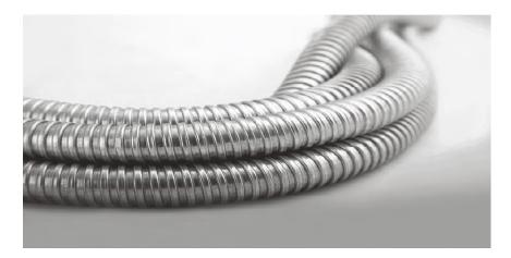
Galvanized steel flexible conduit is suitable for concealed, exposed or approved raceways. The flexible conduit is manufactured with a continuous spiral wound strip of corrosion rust resistant, hot dipped galvanized steel.
